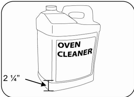
4. Check the degreaser to ensure you have enough to run the AutoClean at the end of the day. If there is less than 3 1/2" left, replace the bottle.
