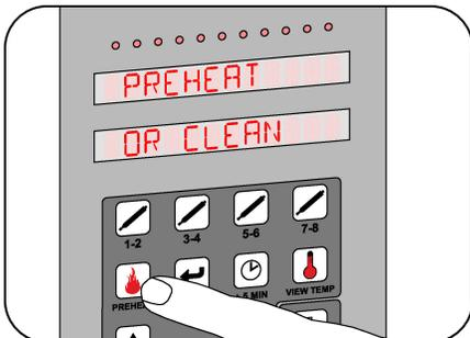
7. Ensure that the water pan is dry. Press the "PREHEAT" button. **DO NOT LOAD UNTIL ROTISSERIE IS PREHEATED.**
