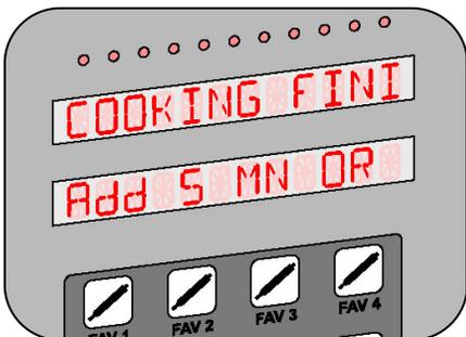
6. At the end of the cooking cycle a buzzer will sound. The display will read "COOKING FINISHED CHECK INT. TEMP". Check temperature of at least 3 of the largest chickens from 3 different skewers before unloading.
