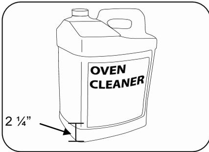
1. Check that the level of degreaser is enough to run the AutoClean. If there is less than 2 1/4" left, replace the bottle.
